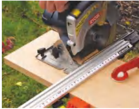
STEP 2. Saw rear and top boards to length, leaving them a tad oversize for cleaning up with a plane
